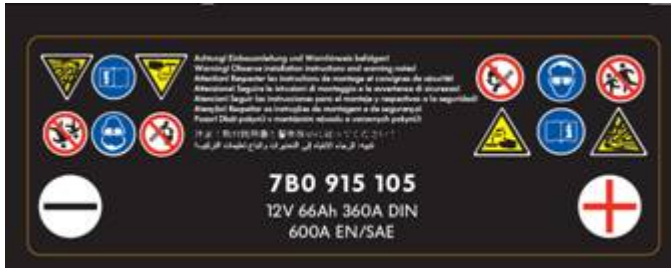
Spare part battery label showing Volkswagen part number, Amp hour, and DIN rating of 360-A.
